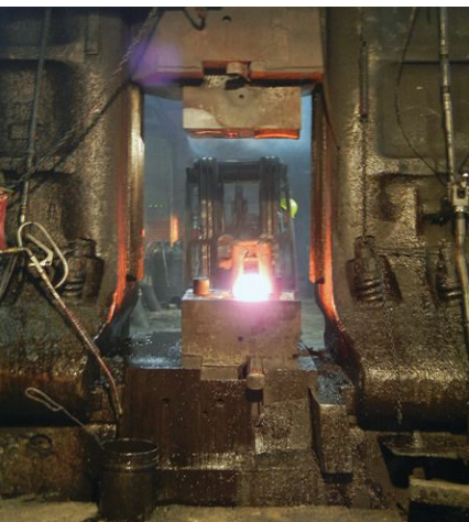
(Left) A forklift positions a heated billet onto the die of the 35,000-pound hammer. (Right) A work associate positions a heated billet on the tooling mounted on the company's 35,000-pound hammer.
