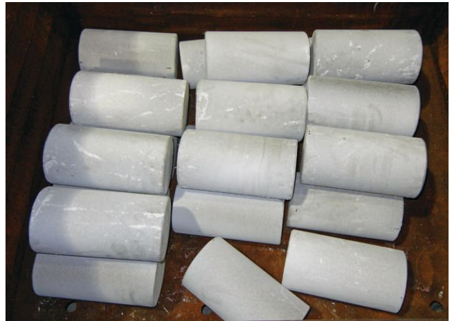
Glass frit is used to coat some billets to prevent unwanted surface oxidation at elevated temperatures.
