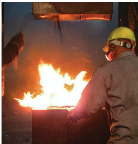
(Left) A forklift positions a heated billet onto the die of the 35,000-pound hammer. (Right) A work associate positions a heated billet on the tooling mounted on the company's 35,000-pound hammer.
