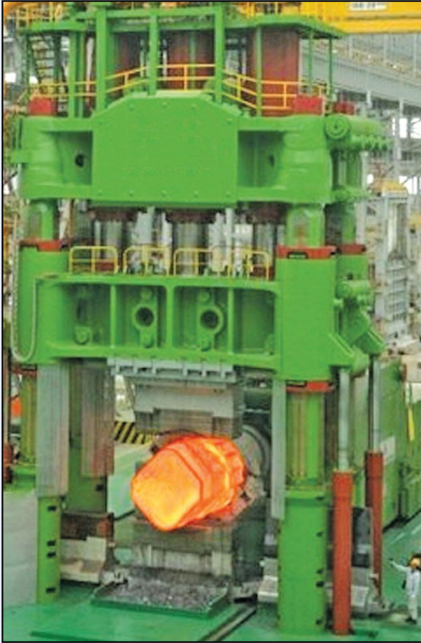
15,000 ton 4-column push down forging a 150 ton ingot
