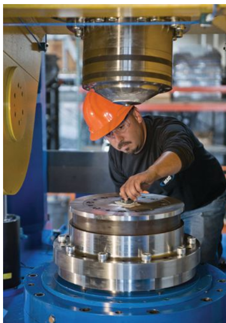
An operator loads a workpiece during a test run on the AFRC machine. Very hard aerospace materials such as Hastelloy and Inconel can be processed by rotary forging.
