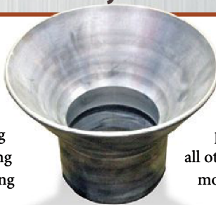
Rotary-forged workpiece shows the flared edge formed by the conical die on the upper spindle.
