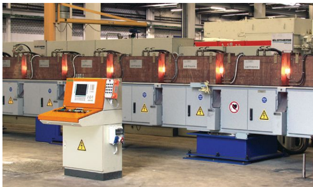
Induction modules are used in series to heat billet material to temperature.
