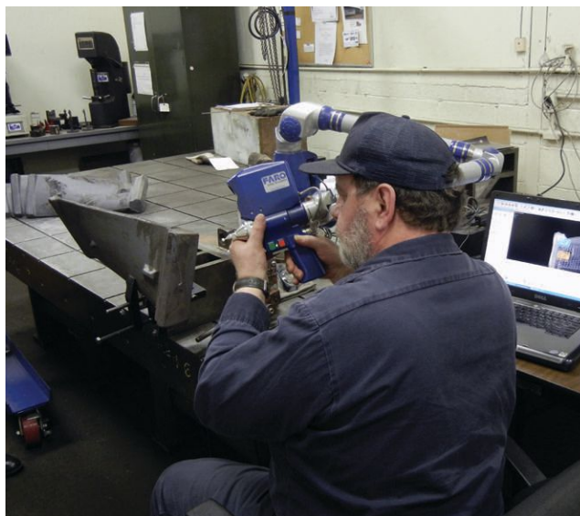
An associate maps and verifies part dimensions according to specification.
